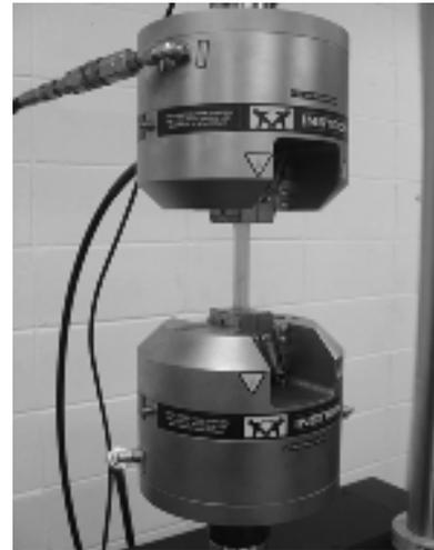
Fig. 2 Tensile test specimen setup with the Instron 8801 test machine
