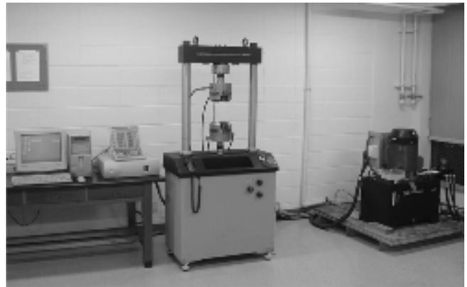
Fig. 7 Test equipment for the grooving process: Instron 8801
